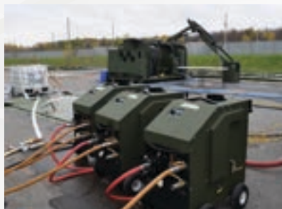
▶ Hot Water Heaters For Military Showers Complete with Stainless Steel Coils. (3 Portable Units)
